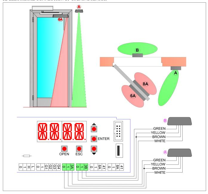
Connect the sensor, using the supplied cable to the terminals of the electronic control as follows:
